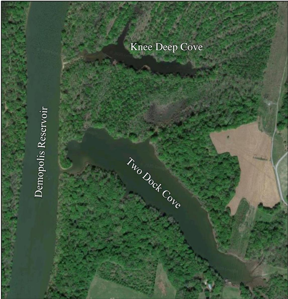
Figure 2. Depiction of a disconnected cove (Knee Deep Cove) and a connected cove (Two Dock Cove) within Demopolis Reservoir, Alabama, due to sediment backfill into the cove mouth (Photo Credit: Google Maps 2020).
