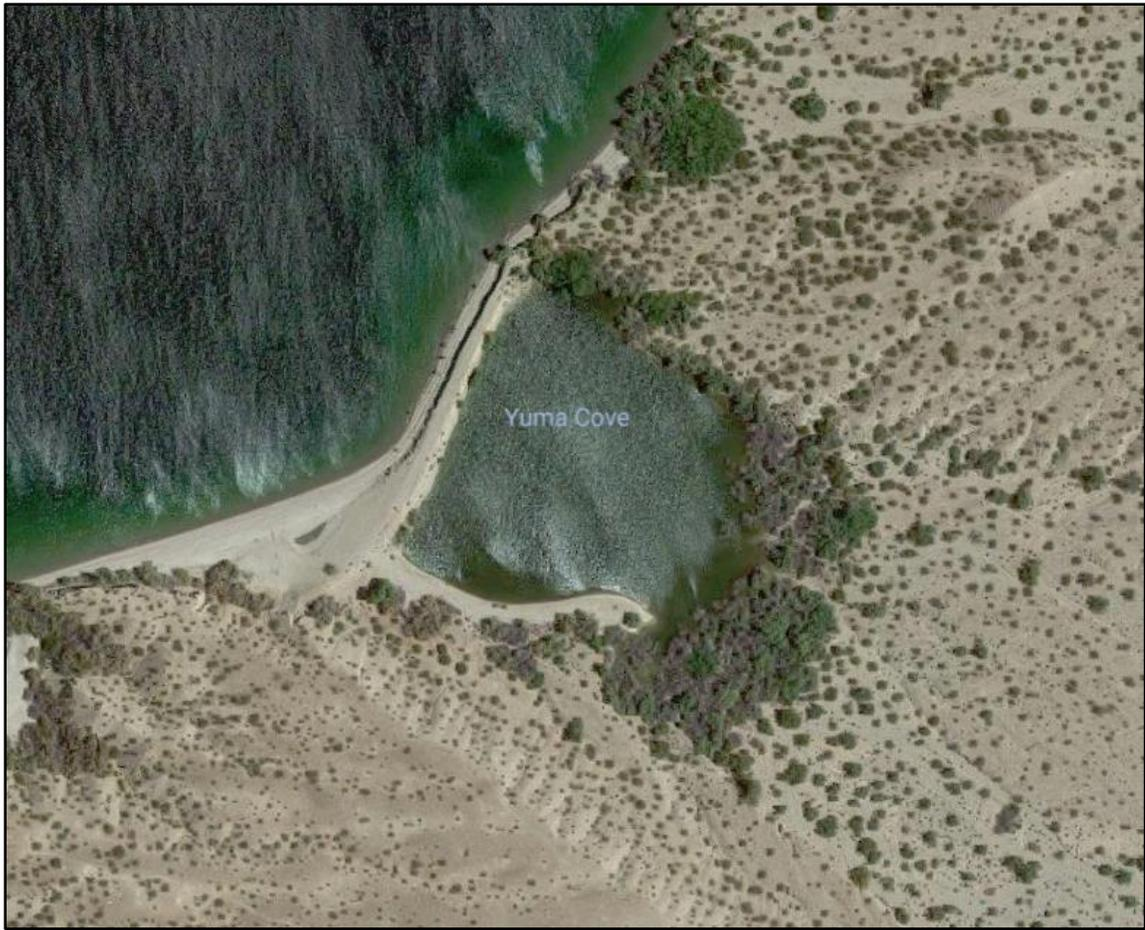
Figure 3. Disconnection of Yuma Cove within Lake Mohave, Arizona, by the formation of a sediment spit due to shoreline erosion and sediment drift (Mueller 1995; Photo Credit: Google Maps 2019).
